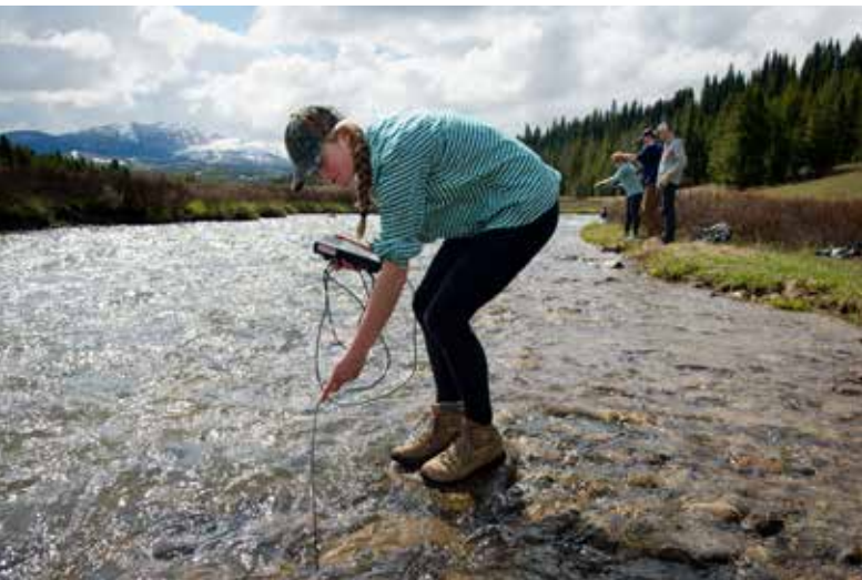
Task Force volunteer, Meredith Hardy, measuring dissolved oxygen at the Big Horn site on the mainstem Gallatin (Figure 1A). Photo credit: Rich Addicks
